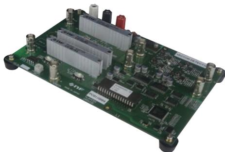
The VD-291 series detects the quadrature phase using The CD-552 series. The amplitude and the phase of the input signal synchronous with a reference signal are calculated by a DSP from the result. That's output as analog voltage.
