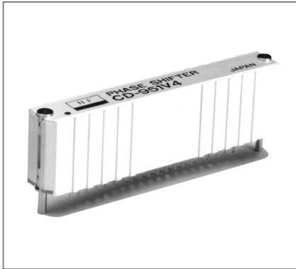
CD-951V4 is a 360°-voltage controlled phase shifter in the frequency range of 1kHz to 2MHz, and adopts CMOS-level (0/+5V) square wave for input and output. This is composed of the ±100°-variable voltage controlled phase circuit and 50%-duty circuit (PAT.P) with 0/180° switch. The combination use of the ±100°-phase shifter and 0/180°-selector enables the output of 50%-duty square wave that phase is shifted in the 360° range to the phase shifter input signal.
